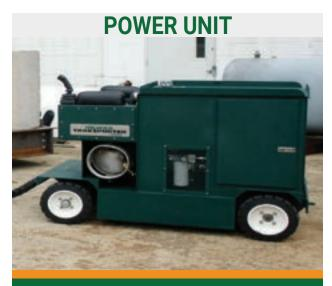
Provides power to the Crawler through a 23hp LPG powered engine that can also be custom designed to run on a 25hp electric motor.
